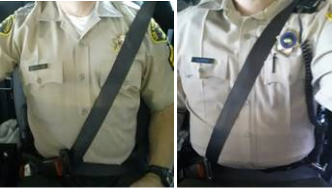
A BAD fit - The buckle is too close to the center of the body.
