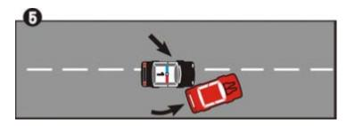
The PIT maneuver causes the rear wheels of the suspect vehicle to break traction, causing it to spin from the rear approximately 180 degrees (figs. 6-9). The deputy must keep a firm, steady grip on their steering wheel
